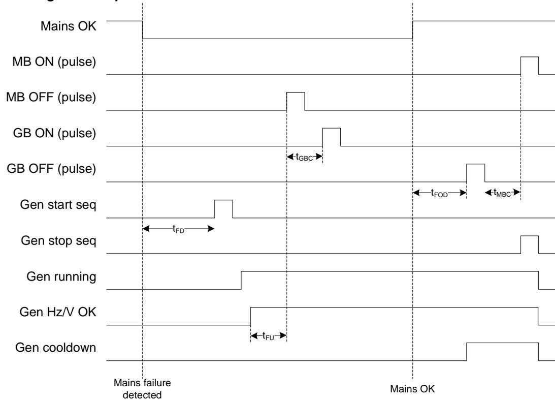
**2 position electrically held, solenoid style ATS or 2 contactors electrically held, (2COEH)**
