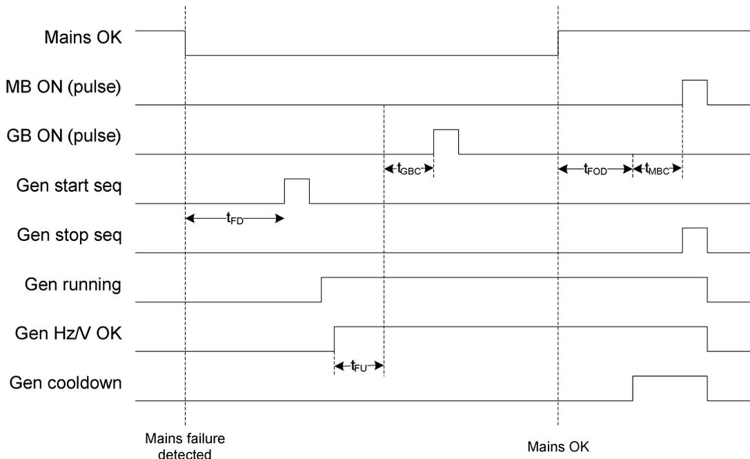
**3 position electrically held solenoid style ATS or contactors (3COEH) – 2 outputs**
