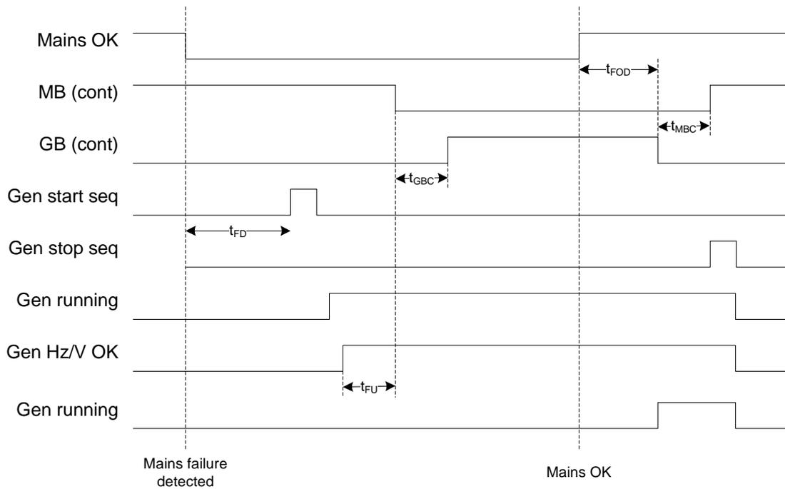
**2 position mechanically held solenoid style ATS or 2 contactors, mechanically held (2COMH)**
