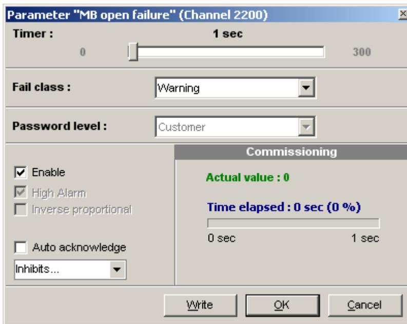
The example below shows the MB close failure timer. If the timer expires before the MB is closed, the alarm will be activated. If no sign signals are used, then the GC-1F will automatically assume that the breaker is closing.
